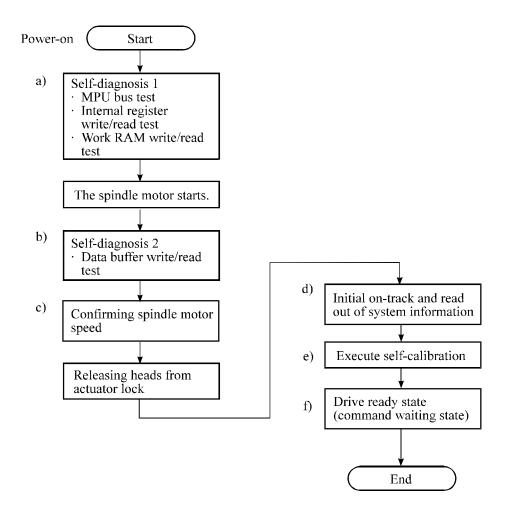
Figure 4.3 Power-on operation sequence
